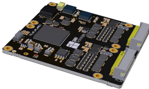
Figure 6: FlashRunner HS NAND Active Module with right-angle device connector
