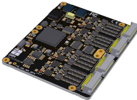
Figure 8: FlashRunner HS GP4 Active Module with right-angle device connectors
